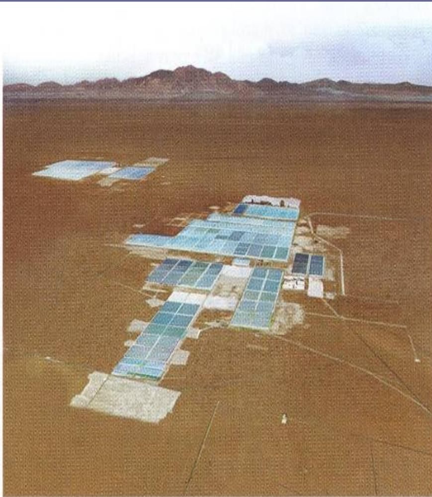
**Figure 10.5** SQM's solar evaporation pond system at the Salar de Atacama covering an area equivalent to 7000 football pitches and in excess of 30 km<sup>2</sup>. (Photograph courtesy of Sociedad Quimica y Minera de Chile S.A. (SQM).)
